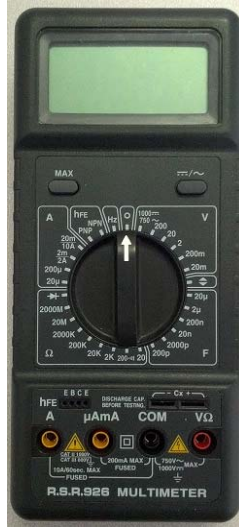
Figure 4. Digital multi-meter (DMM) used for making electrical measurements.
